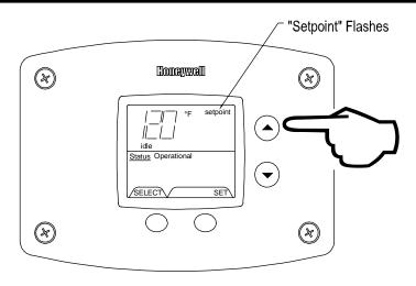
Step 4: To lower the temperature setpoint, press the "Temperature Down" button until the desired temperature is shown on the water heater display.
